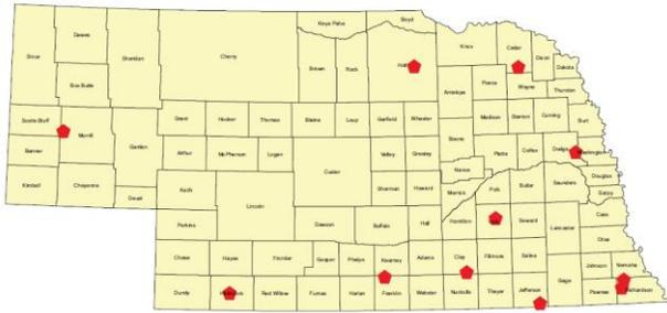
Figure 4. Public water supplies on administrative order for nitrate-nitrite concentrations above 10 mg/L in 2011 (NDEQ, 2012).
