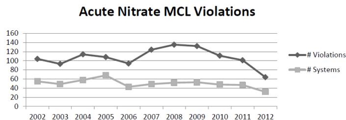
Figure 3. Number of public water systems and acute violations with nitrate concentrations in excess of 10 ppm in Nebraska (NDHHS, 2012).
